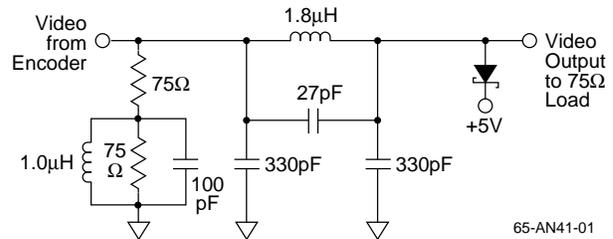
**Figure 1. Video Output Filter with Latchup Protection Diode**
